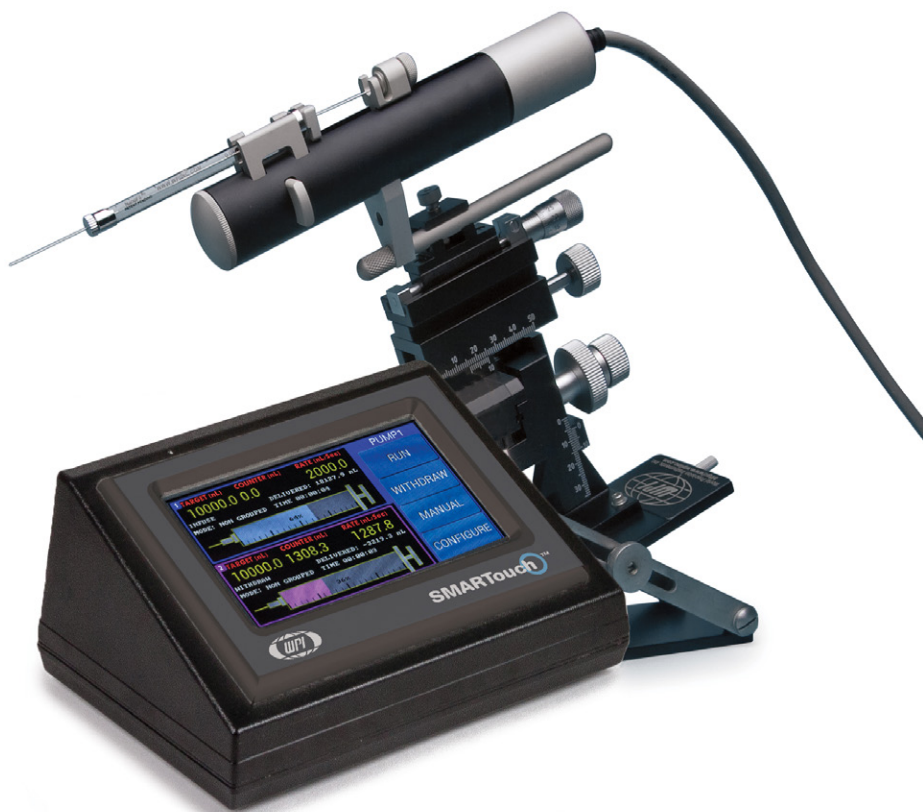
Fig. 1—The MICRO2T SMARTouch™ controller is a touch screen controller for use with the UMP3 and Nanoliter series pumps. The UMP3 shown here is mounted on WPI's M3301 micromanipulator and TB-1 stand (not included). Mounted on the UMP3 is our signature NanoFil™ syringe (not included).
