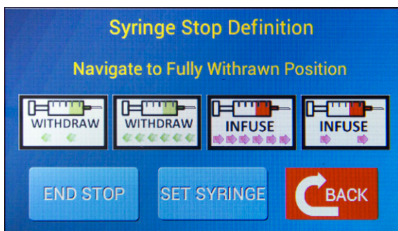
Fig. 17—The Syringe Stop Definition screen lets you define the limits of travel for the pump.
