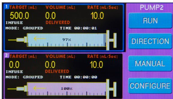
Fig. 38—Pump 2 is the Master pump, and Pump 1 is the slave in this example.
