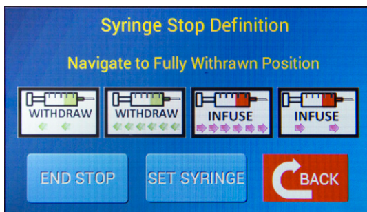
Fig. 18—The Syringe Stop Definition screen has four white navigation buttons used to position the syringe plunger when defining travel limits.
