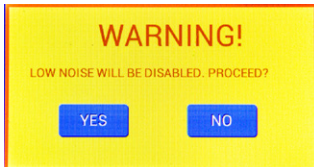
Fig. 24—Warning message appears to let you know that the motors will be re-engaged and the Low Noise Recording period will end.
