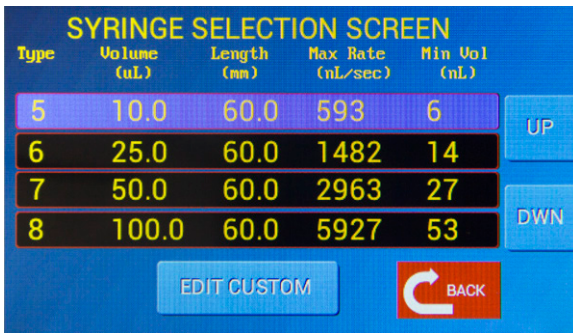
Fig. 27—You can define custom syringes using the Syringe Selection screen. Select one of the three user-defined syringe types—A, B or C.
