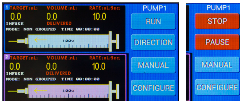
Fig. 31—Use the Command screen to control the pumps.
